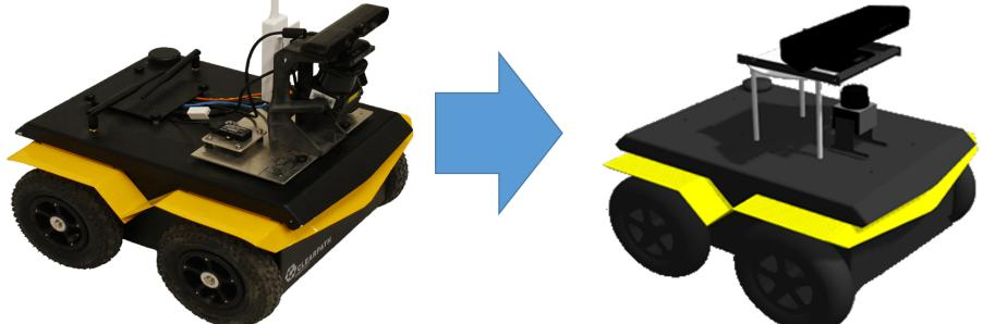
High-Fidelity Virtual Clearpath Robotics Jackal equipped with same sensors as physical platform
